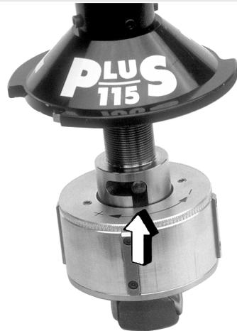
4. Before engaging the lead screw, it must be rotated to the full length by hand. Engage the lead screw onto the collaring head so that the drive pin of the shank is in the groove of the lead screw.
