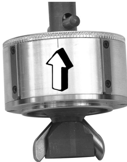
4. Rotate the cover plate relative to the cylindrical cover clockwise for increasing and counter-clockwise for decreasing the diameter of adjustment. One notch on the cover plate equals to 0.5mm / 0.02" on the forming pin span.
