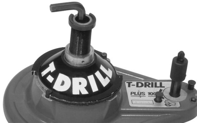
2. Loosen the 4 screws of the knurled handle of the lead screw with 4 mm hex wrench and remove the handle.
