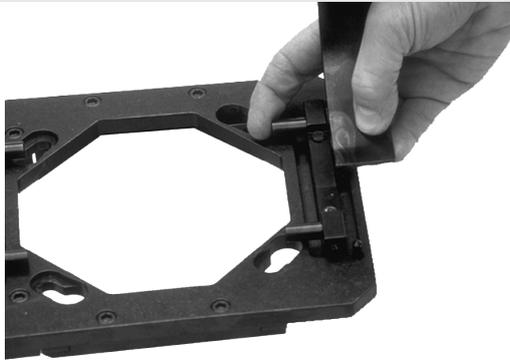
1. Choose the ring clamps according to the run tube diameter and fix the clamps to the base plate. Attachment takes place with the clamp locking pins in the base plate.
