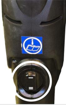
6. Turn the speed selector knob on the T-65 to position I. You may have to “pump” the foot pedal to get it engaged.
