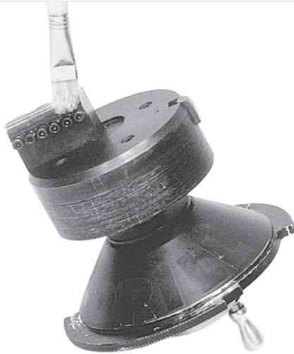
2. Lubricate the facing tool blade.
