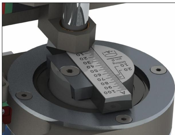
The A and B dimensions of the ellipse are adjusted by loosening the locking screws (Adjust scales separately, so that the locking screws are open only one at a time). The adjustment is done by sliding the scale in the desired direction. The diameter of the milling pin is screened on the same line as the desired dimension and tightening the screw. The best size of the milling pin is proved to be 11.3mm.
